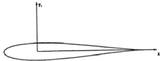
Figure 4. Schematic of a Joukowski Airfoil
