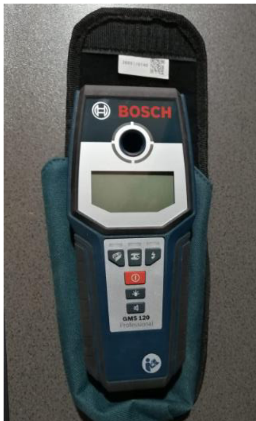
Figura 29. Detector de materiales BOSCH GMS 120 Professional
