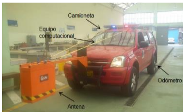
Figura 8. Ground Penetrating Radar (GPR)
