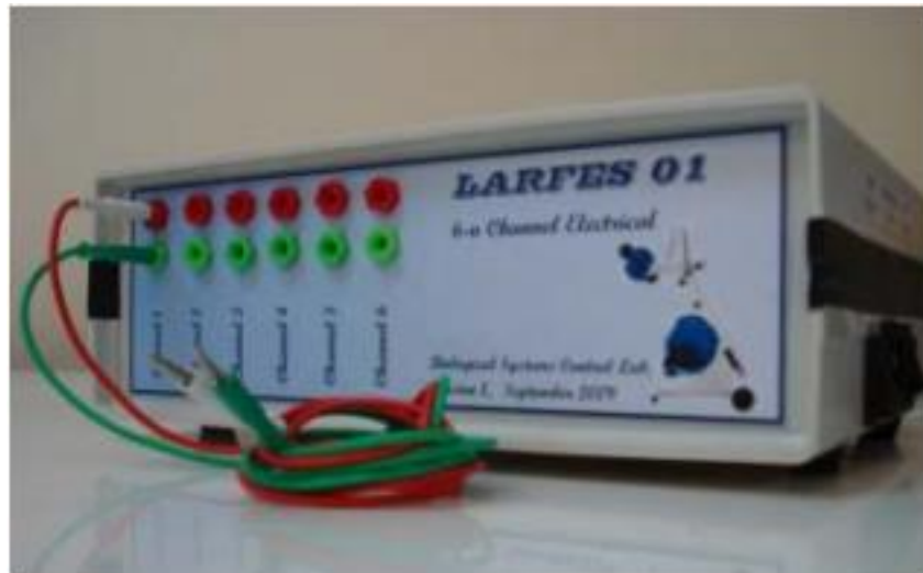
Figura 11: The front view of the device. Each pair of colors represents one output channel.
