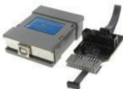
**Figura 78: Programador Cross Connect (JTAG)**
